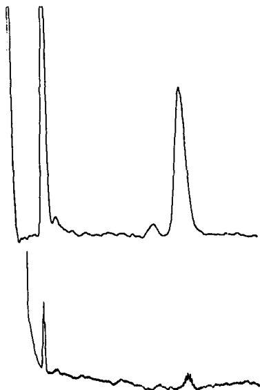
Fig. 7. Illustration of the enhancement of signal-to-noise ratio. The lower chromatogram shows a direct display, the upper chromatogram that after solute switching and synchronous demodulation. Sample, 5 ml of clean air.
